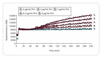
Kinetic determination of antigen-antibody binding at different concentrations.<sup>3</sup>
