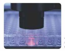
Insoluble particles in solution in a microplate well scatter laser light
