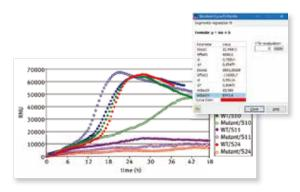
The MARS data analysis software provides sophisticated tools for automated data reduction.
