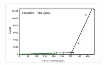
Solubility screen of hydrocortizone. The intersection at 310  $\mu g/L$  indicates the point of precipitation.<sup>1</sup>
