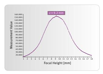
The automated focal height adjustment ensures the best signal-to-noise ratio in all detection modes and all plate formats.
