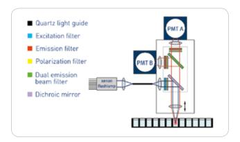
Schematic layout of the Simultaneous Dual Emission optical pathway incorporated in the PHERAstar FSX.
