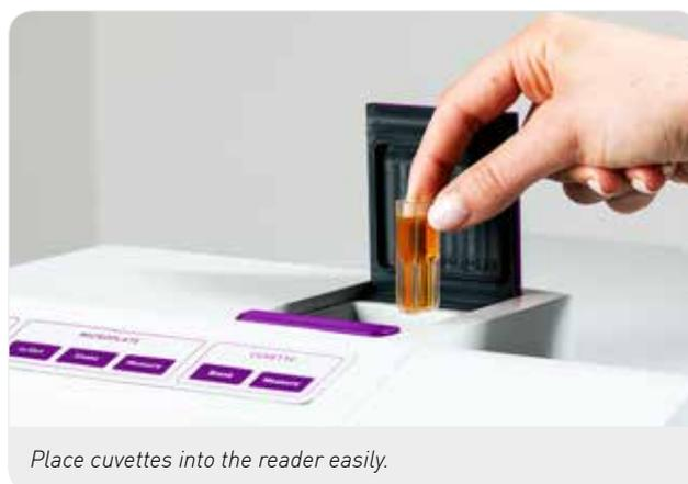
Place cuvettes into the reader easily.
