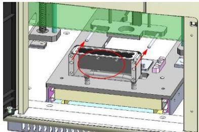
[Inserting two holding shafts (red arrows) into the Tip Protector]
