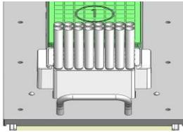
(6) Place the Disposable tip rack on the base plate.
