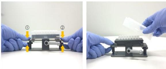
(Picture of pressing down each side of Separation Tool and removing Protection Cover from Separation Tool)
