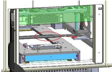
[Placing the Contamination Shield on the projecting part (red arrow)]
