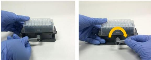
(Picture of lever rotation for fixing Elution Tube Rack to Protection Cover Separation Tool)
