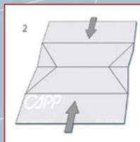
*Push the two outer sides against the middle to flick the CappOrigami™ reservoir into shape.*
