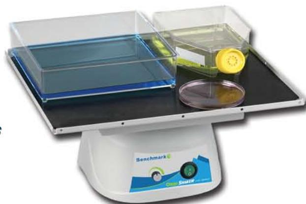
The Orbi-Blotter features a gentle orbital motion with speed control down to as little as 3 rpm, making it the ideal orbital choice for low speed applications, such as blotting, washing, staining/destaining, etc. A large 14x12 in. platform is included along with a non-slip rubber mat for holding trays, dishes, plates, flasks and other flat bottomed vessels. An optional stacking platform is also available for protocols requiring an increased work surface.
