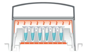
When the ThermoTop is placed on the device, it begins heating immediately. The temperature optimally adapts to the test temperature to ensure that it does not negatively affect the sample. Condensation droplets have no opportunity to form.
