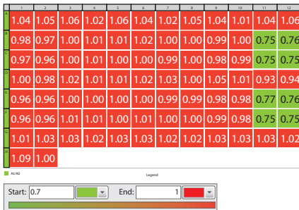
Fig. 3: BRET1 ratio values obtained with the CLARIOstar. A color gradient was applied using green to indicate a successful ligand binding and red to show a negative result.
